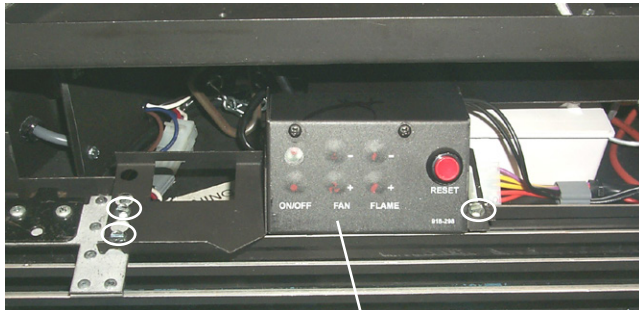
Manual Control Box
